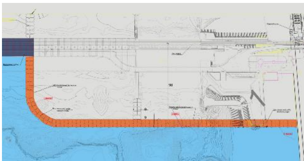
Fig.6 Reconstruction of the Kakhovka HPP. Temporary dam from the downstream side.
