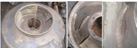
Fig.2 Double flux impeller and damages on it.
